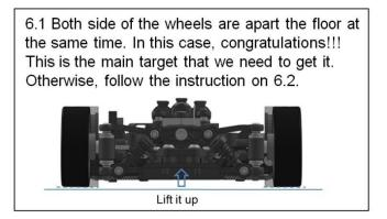
6.2 One of the wheel apart the floor first. For example, if the **left** wheel apart first, adjust the **right** side damper (above the motor) in adding the shim (SM6) until both wheels apart the floor like 6.1. If the right wheel rise up first, do the same on other side.
